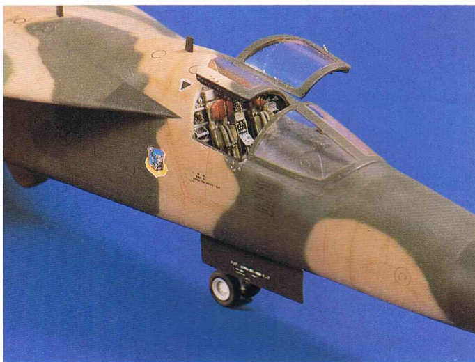
Inside detail of the canopy doors can be found in the VP kit in the form of photo-etched parts which have to be folded and shaped before glueing.
