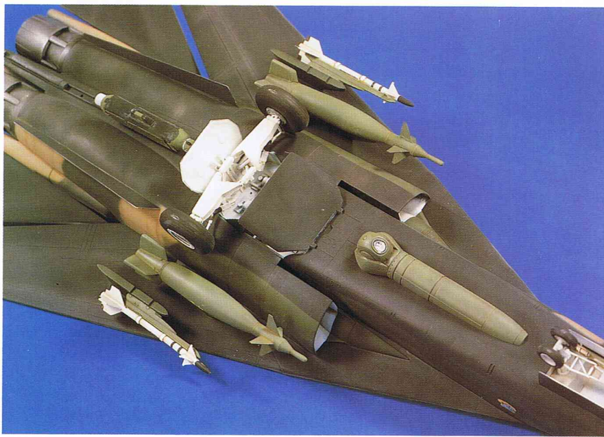
The various VP parts seen mounted on the F-111 belly. The Pavetack laser guiding system, the AN-ALQ131 jamming pod, the Sidewinder missiles and the Paveway laser guided bombs.
