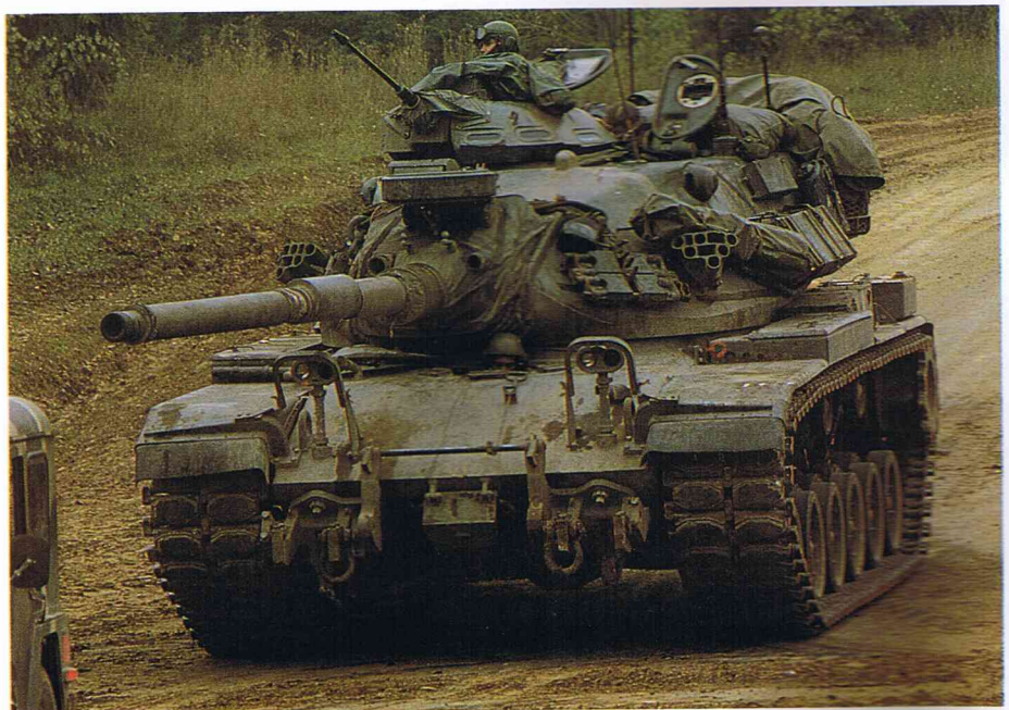
An M60A3 CEV at the Hohenfels Training Grounds in Germany. The spade mounting brackets are clearly visible. Also apparent are the elevated headlights with guards and the control valve manifold assembly in the center of the front hull plate.
