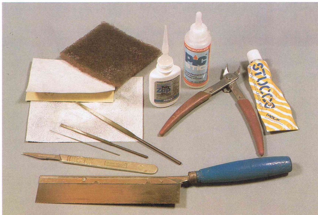
Fig.1 The proper tools to handle resin carriers. A sharp knife with a new blade, an X-acto handsaw and flush cut nippers to remove the carriers from the parts ; files, sandpaper and some Scotch Brite to clean the surfaces. The tube of filler and some super glue (two brands shown) are used to assemble the various parts of the figure.
