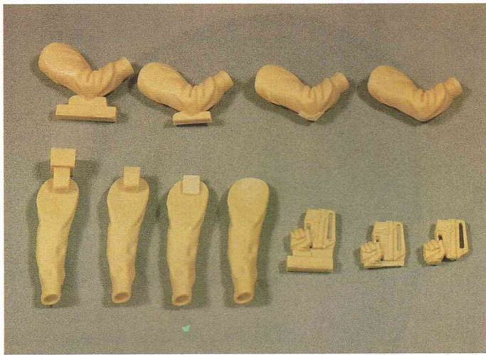
Fig.2 A layout of some different figure parts, showing the subsequent removal of the secondary and primary carrier. The final part has been cleaned thoroughly with Scotch Brite.
