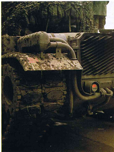
The installation of the fluid reservoir on the rear left fender (after removal of part of the mudguard) before (above) and after the complete tube assembly had been installed (below right).
